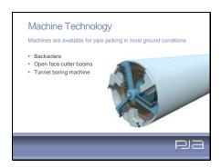
A tunnel boring machine – a shield having a rotating head. Various cutting heads are available to suit a broad range of ground conditions.
