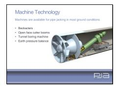
An earth pressure balance machine or EPBM – a full-face tunnel boring machine in which the excavated material is transported from the face by a balanced screw auger or screw conveyor. The face is supported by excavated material held under pressure behind the cutter head in front of the forward bulkhead. Pressure is controlled by the rate of passage of excavated material through the balanced screw auger or valves on the screw conveyor.
