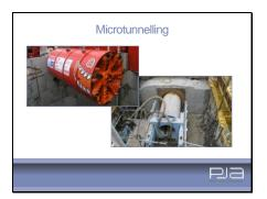
In smaller non-man entry diameters, generally one metre and below, the system is often referred to as microtunnelling although this term is also used to describe automated tunnelling operations in larger diameters.
