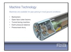
A slurry machine - another full-face tunnel boring machine in which the excavated material is transported from the face suspended in a slurry. Various cutting heads are available to suit a broad range of ground conditions and may incorporate internal crushers to deal with cobbles and small boulders. The pressure of the slurry is used to balance the groundwater and face pressure.
