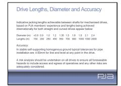
Tunnelling technology enables mechanised drives up to a kilometre or greater to be undertaken depending on pipe diameters. When operatives are working within the tunnel a risk analysis must be undertaken to ensure all hazards are assessed to include access and egress. In stable, self-supporting homogenous ground, typical tolerances for pipe installation are ±50 mm of line and level.
