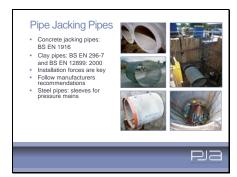
A range of materials are used as pipe jacking linings to include concrete, grp, clay and steel. Concrete jacking pipes which usually incorporate reinforcement, and have flexible joints, and clay pipes, should be manufactured in accordance with relevant standards.
