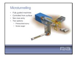
These fully guided machines are remotely controlled from the surface. There are generally two types, both having face support capability, pressurised slurry and auger machines.
