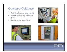
Guidance systems linked to an operator console enable continual line and level checks. Far greater control of accuracy and tolerance compliance is ensured even in the most difficult ground. The requirement for man-entry into the pipejack is minimised with surveying operations managed from the surface.
