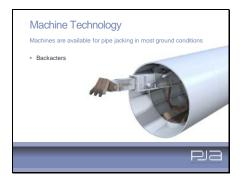
A backacter – an open face shield in which a mechanical backacter is mounted for excavation purposes.
