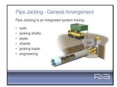
The integrity of a pipe jacking operation is dependent upon the inter-relationship of a number of factors: soil investigation and interpretation; jacking shaft design; pipe design; pipejack shield selection; hydraulic considerations; and laser engineering and control.
