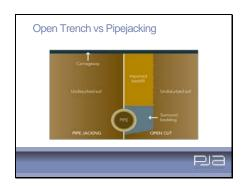
Comparing open-cut with pipejacking it shows that disruption is largely eliminated. The requirement for excavation is dramatically reduced as there is no requirement for imported fill.
