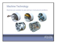
The latest tunnelling technology has been incorporated into pipe jacking excavation systems and a range of machines are available for pipejacking in most ground conditions from soft water bearing strata to hard rock.
